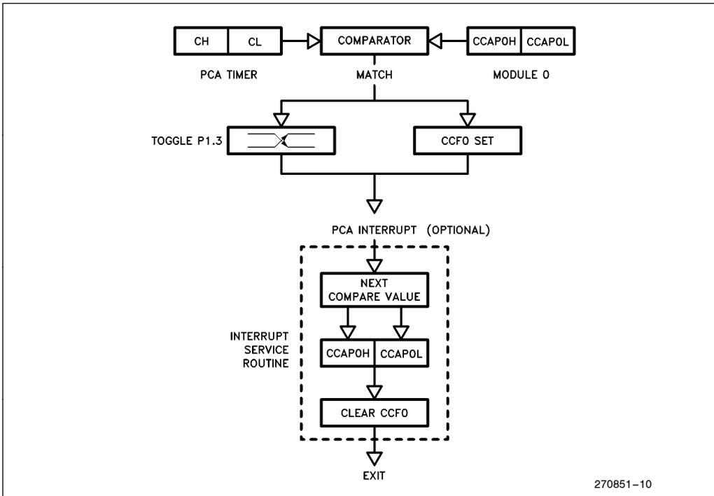
**Figure 10. High Speed Output Mode (Module 0)**
