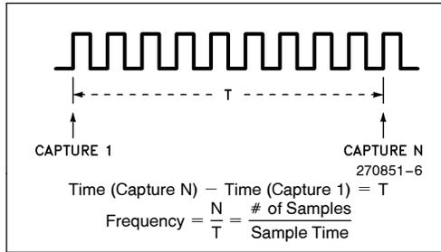
**Figure 6. Measuring Frequency**
