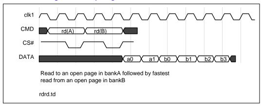
Figure 28. Multibank Timing Relationship Diagram B
