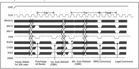
Figure 5. Power Up Initialization Sequence
