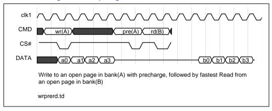
Figure 41. Multibank Timing Relationship Diagram O
