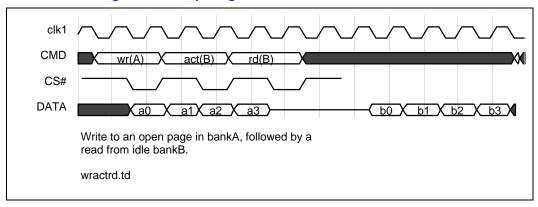
Figure 34. Multibank Timing Relationship Diagram H
