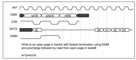
Figure 43. Multibank Timing Relationship Diagram Q
