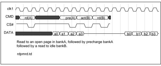
Figure 35. Multibank Timing Relationship Diagram I
