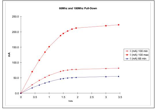
Figure 55. SDRAM DQ Output Buffer Pull-Down Characteristics
