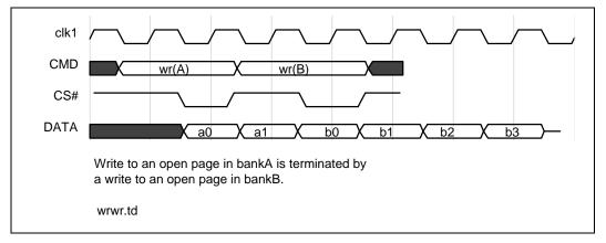
Figure 31. Multibank Timing Relationship Diagram E
