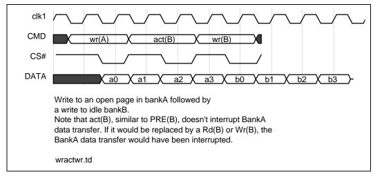
Figure 32. Multibank Timing Relationship Diagram F
