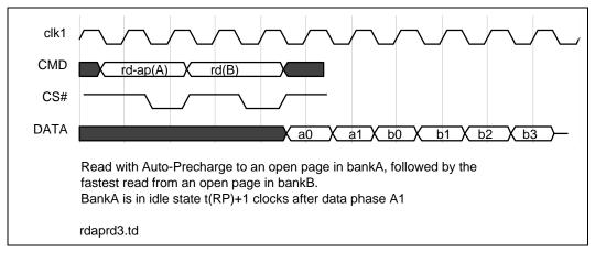
Figure 49. Multibank Timing Relationship Diagram W
