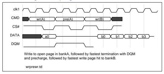
Figure 40. Multibank Timing Relationship Diagram N
