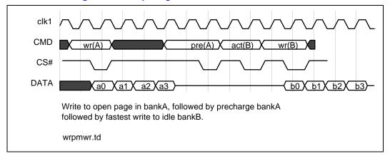
Figure 38. Multibank Timing Relationship Diagram L
