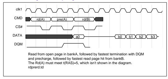
Figure 37. Multibank Timing Relationship Diagram K
