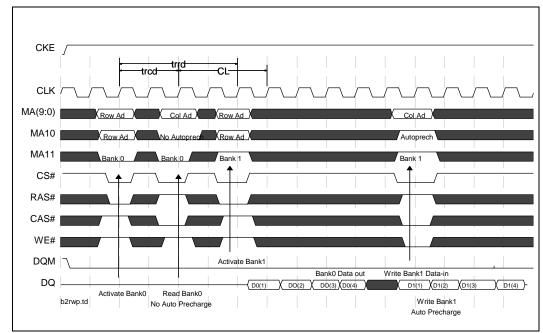
Figure 8. Read and Write Commands (Burst Length 4 Shown)
