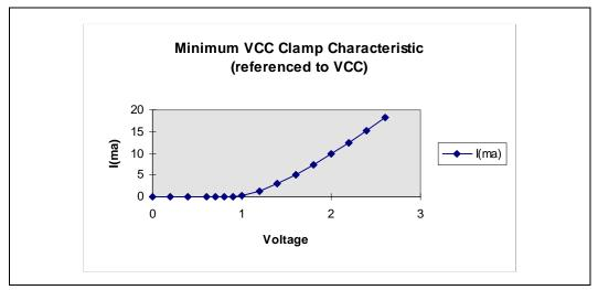
**Figure 54. SDRAM VCC Clamp Characteristics**
