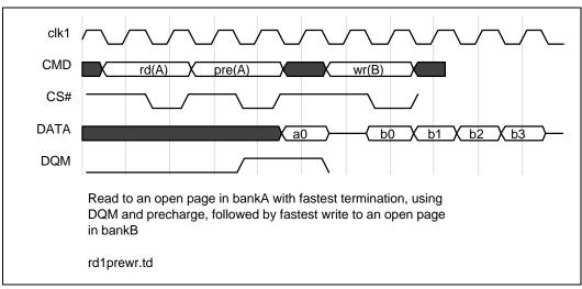
Figure 46. Multibank Timing Relationship Diagram T
