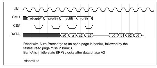
Figure 47. Multibank Timing Relationship Diagram U
