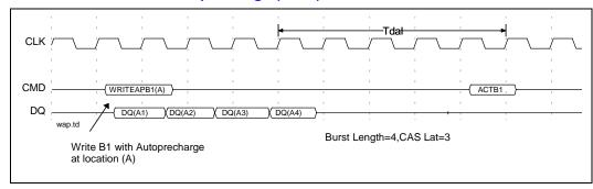
Figure 21. Write Command With Autoprecharge (BI=1)
