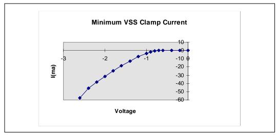
Figure 53. SDRAM VSS Clamp Characteristics
