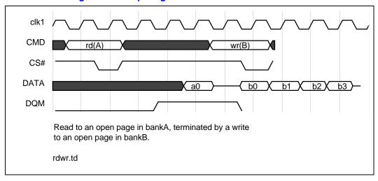
Figure 29. Multibank Timing Relationship Diagram C
