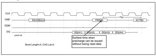
Figure 10. Precharge Command After Burst Read
