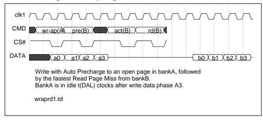
Figure 50. Multibank Timing Relationship Diagram X
