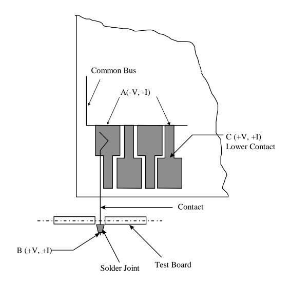
Figure 10: Electrical Testing Schematic
