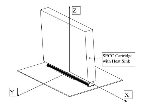
Figure 13: Schematic of Axes Orientation for Vibration Test
