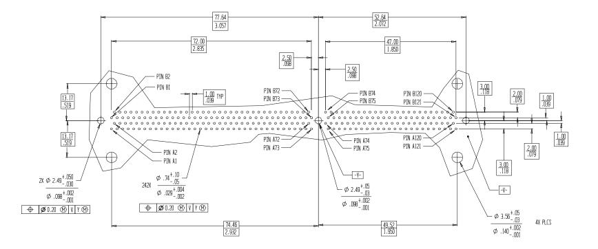
**Recommended clearances around 3.56 mm DIA (0.140 inch DIA) mounting Holes:**
