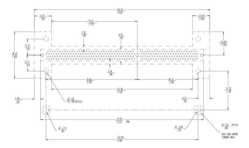
Figure 6: Mechanical Keep-Out Area Around Connector
