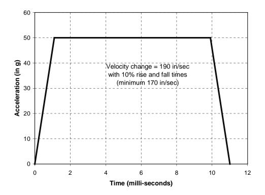
Figure 15: Shock Pulse Curve
