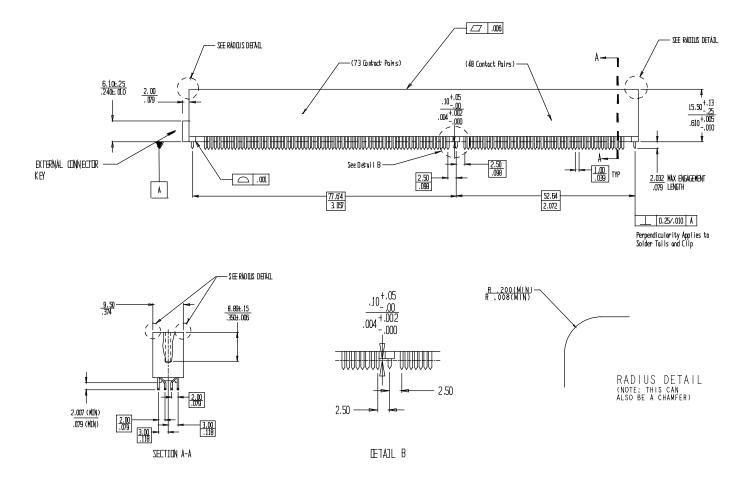
**Figure 4: Connector Dimensions**
