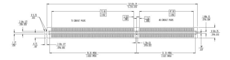
Figure 5: Connector Dimensions, con't.
