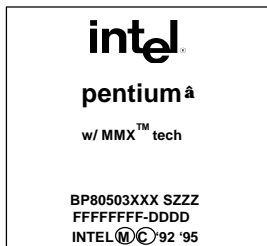
xB1-Step Boxed Pentium® Processor w/MMX™ Technology Production SPGA Units:
