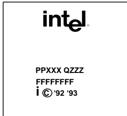
mcC0-Step Engineering Sample TCP Units:
