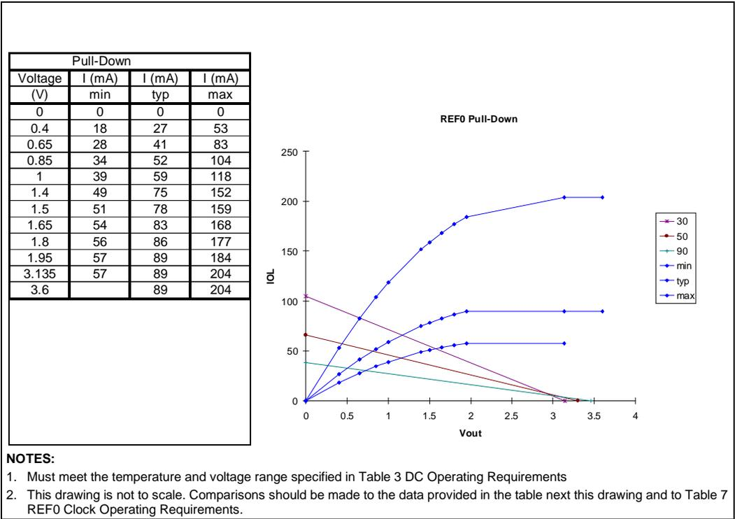
Figure 8. TYPE 4: REF0 Clock Output Buffer Pull-Down Characteristics
