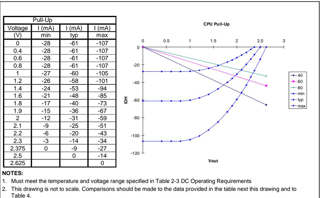
Figure 1. TYPE 1: CPU Clock Output Buffer Pull-Up Characteristics
