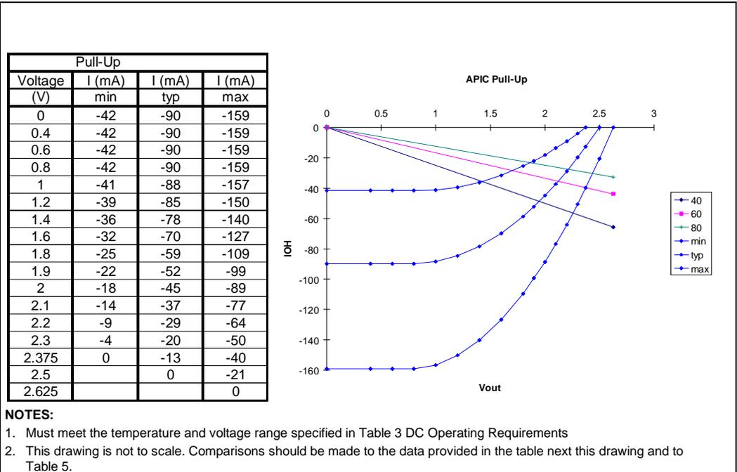
**Figure 3. TYPE 2: IOAPIC Clock Output Buffer Pull-Up Characteristics**
