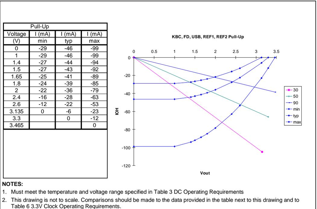
Figure 5. TYPE 3: 3.3V Clock Output Buffer Pull-Up Characteristics
