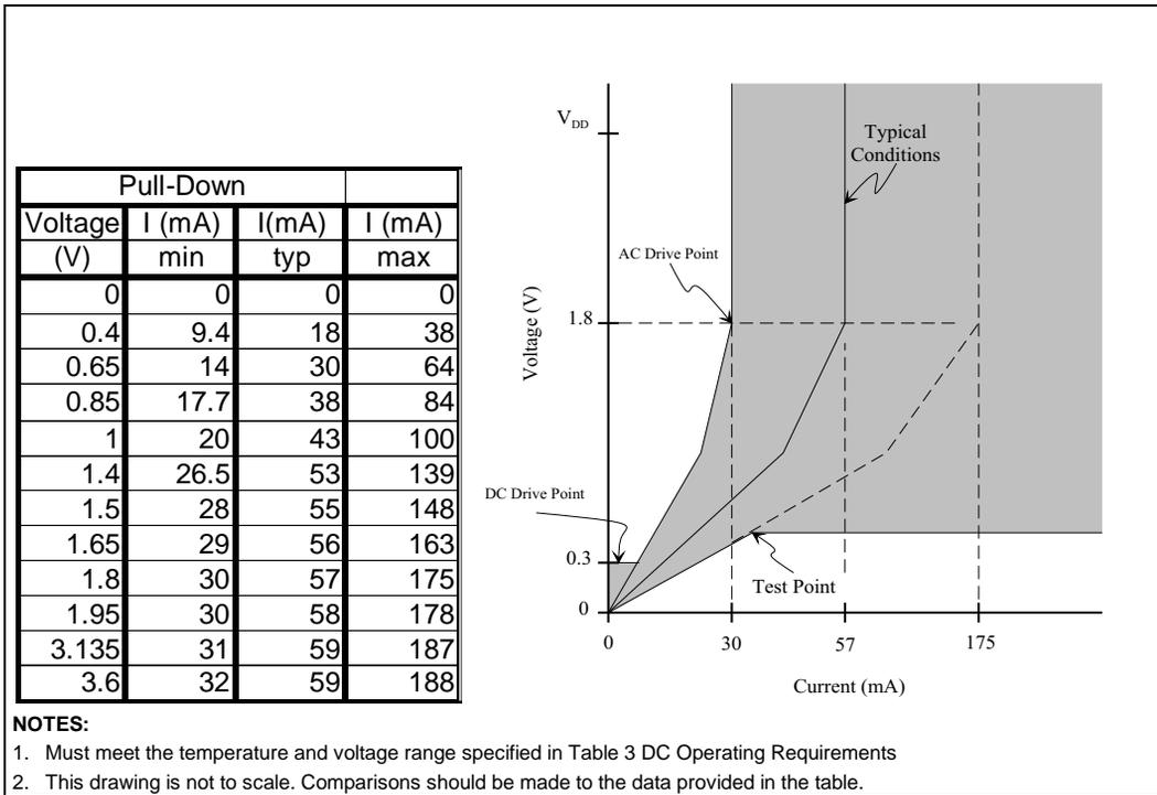
**Figure 10. TYPE 5: PCI Clock Output Buffer Pull-Down Characteristics**
