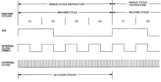
Note that changing the clock divisor, either manually or through a switchback, will not affect Timed Access procedures. Timed Access operates in relation to internal machine cycles, not an absolute time reference.
