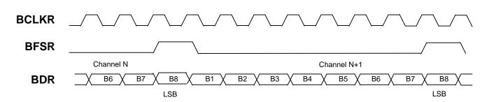
Note that in Figure 4, the Receive synchronization pulse BFSR occurs at the LSB of each timeslot of the DS21x52 transmit datastream. The requirements needed for this signal is very much like the RCHCLK signal of the DS21x5y, with the exception of the 24<sup>th</sup> timeslot. Like the transmit side, this exception will cause some external logic requirements to be implemented to ensure proper operation.
