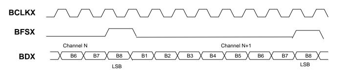
Note that in Figure 3, the Transmit synchronization pulse BFSX occurs at the LSB of each timeslot of the DS21x52 transmit datastream. The requirements needed for this signal is very much like the TCHCLK
