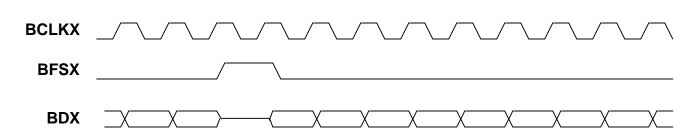
Note that in Figure 1, the Transmit synchronization pulse occurs at the location where the DS21x5y inserts a frame bit. Since the DS21x5y will internally generate the frame bit, and the '54x is not using the bit position where a frame synchronization pulse occurs, this allows a glueless interface between these two devices on this signal.
