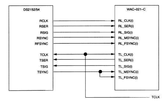
In the circuit shown above the framer outputs a multi-frame synchronization pulse on TSYNC. The signal drivers both TL\_FSYNC and TL\_MSYNC of the WAC-021-C. TL\_FSYNC does not need to be driven at every frame boundary. TSYNC may be programmed as an input if the user wishes to define multiframe boundaries or slave several devices to the same multi-frame/ frame boundary.
