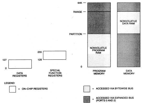
NOTE: Partitionable mode is not supported when MSEL pin = 0 (128kB mode).
