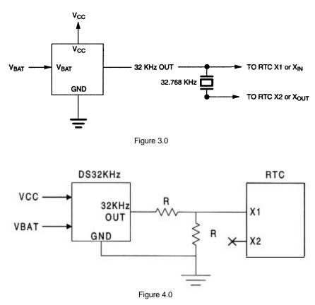
Figure 3.0 illustrates how a standard 32.768 kHz crystal and the DS32KHz should be connected to address the interchangeable option. Using this connection scheme and the recommended layout provides a solution which requires no hardware modifications. Only one device should be used at a time and both layouts should be located very close together if the recommended layout is not used.
