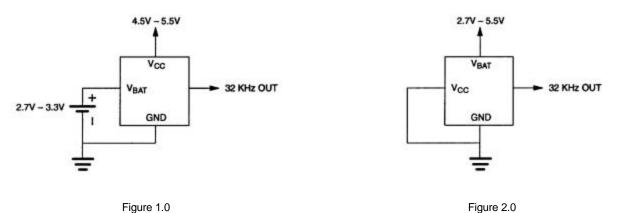
Figure 1.0 shows how the DS32KHz should be connected when using two power supplies.  $V_{CC}$  should be between 4.5 and 5.5 volts while  $V_{BAT}$  should be between 2.7 and 3.3 volts. Figure 2.0 shows how the DS32KHz can be used when only a single supply system is available.  $V_{CC}$  should be grounded and  $V_{BAT}$  should then be held between 2.7 and 5.5 volts. The  $V_{BAT}$  pin should be connected directly to a battery using no external components.
