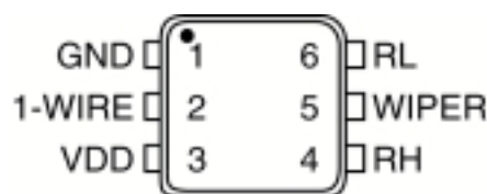
6-pin TSOC (top view)
