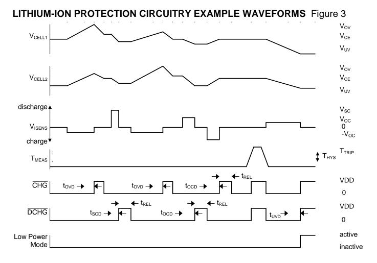
**Summary.** All of the protection conditions described above are ORed together to affect the  $\overline{CHG}$  and  $\overline{DCHG}$  outputs. Taking the OV, UV and OT bits from the Status Register and considering the OC Status Register bit to be the logical OR of DOC (discharge overcurrent) and COC (charge overcurrent), the equations for  $\overline{CHG}$  and  $\overline{DCHG}$  are as follows:
