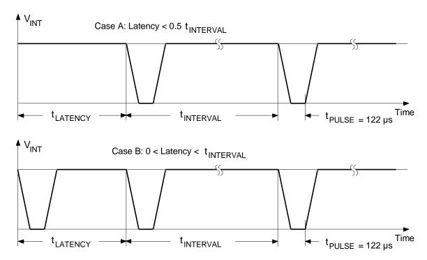
The latency depends on the selected interrupt interval (ISO to IS2 settings) and the contents of the RTC counter at the time of writing the device control byte. In Case A, the flip-flop that determines the interval duration is reset and toggles before half of the interval time is over. In Case B, this flip-flop is set which generates an immediate interrupt pulse; the latency, therefore, can be up to one full interval duration.
