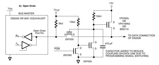
The interface is reduced to the  $5k\Omega$  pull-up resistor if one does not intend to program the EPROM cells.
