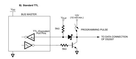
The diode and Programming Pulse circuit are not required if one does not intend to program the EPROM cells.
