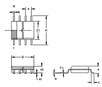
The chamber on the body is optional. If it is not present, a terminal 1 identifier must be positioned so that  $\frac{1}{2}$  or more of its area is contained in the hatched zone.
