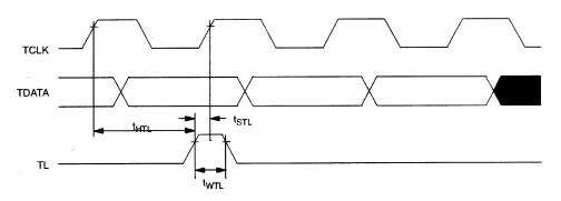
NOTE: The rising edge of TL causes the internal pattern generation circuitry to be reloaded; the first bit of the new pattern (the shaded one) will appear after two TCLK periods.
