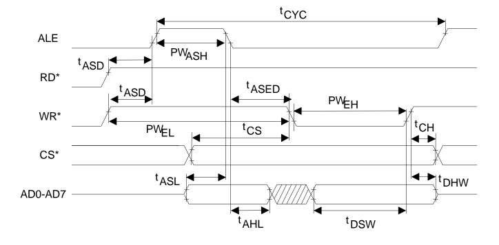
Figure 24-3 MOTOROLA BUS TIMING (BTS = 1 / MUX = 1)
