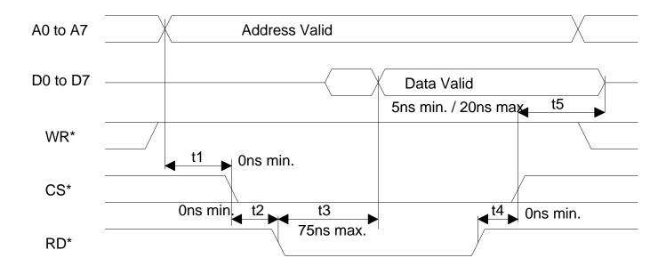
Figure 24-5 INTEL BUS WRITE TIMING (BTS=0 / MUX=0)
