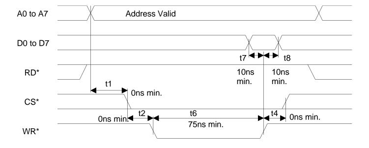
Figure 24-6 MOTOROLA BUS READ TIMING (BTS=1 / MUX=0)
