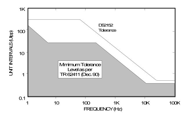
Figure 16-5 JITTER ATTENUATION
