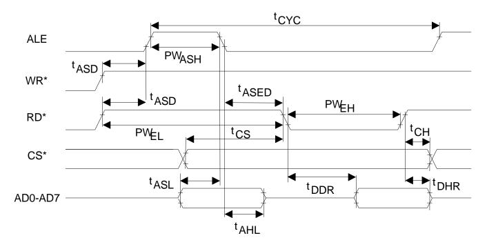
Figure 24-2 INTEL BUS WRITE TIMING (BTS=0 / MUX=1)
