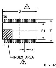
DIMENSIONS D AND E1 INCLUDE MOLD MISMATCH, BUT DO NOT INCLUDE MOLD FLASH, PROTRUSIONS OR GATE BURRS. MOLD FLASH, PROTRUSIONS OR GATE BURRS SHALL NOT EXCEED 0.254 MM PER SIDE.
