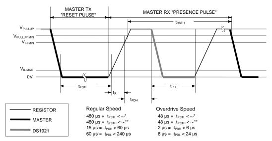
$^{*}$  In order not to mask interrupt signalling by other devices on the 1-Wire bus,  $t_{\text{RSTL}}$  +  $t_{\text{R}}$  should always be less than 960  $\mu s$
