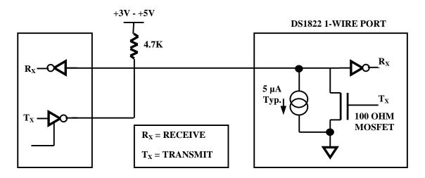
The idle state for the 1–Wire bus is high. If for any reason a transaction needs to be suspended, the bus MUST be left in the idle state if the transaction is to resume. Infinite recovery time can occur between bits so long as the 1–Wire bus is in the inactive (high) state during the recovery period. If this does not occur and the bus is left low for more than 480 µs, all components on the bus will be reset.
