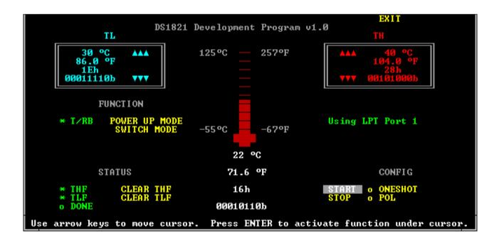
The DS1821K Programmable Digital Thermostat Development Kit allows a potential user of the DS1821 to observe the operation of the DS1821 in an actual temperature measurement application. Temperature is measured and displayed in a text box, as well as on a graphical thermometer.
