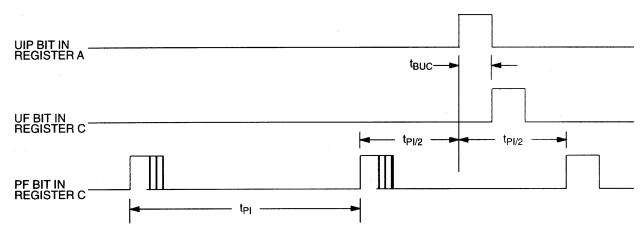
$t_{Pl}$  = PERIODIC INTERRUPT TIME INTERNAL PER TABLE 1  $t_{BUC}$  = DELAY TIME BEFORE UPDATE CYCLE = 244  $\mu s$
