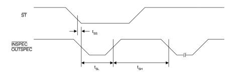
NOTE: INSPEC/OUTSPEC generate a total of four low pulses.
