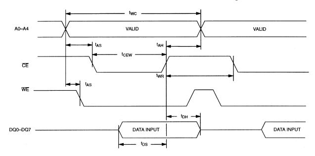
**BURST MODE TIMING CHARACTERISTICS** (0°C to 70°C; V<sub>CCI</sub>=5.0V±10%)
