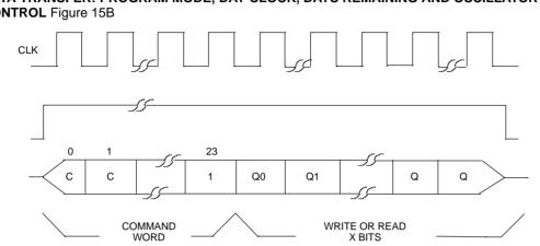
DATA TRANSFER: PROGRAM MODE, DAY CLOCK, DAYS REMAINING AND OSCILLATOR CONTROL Figure 15B
