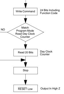
SEQUENCE: PROGRAM MODE, READING THE 20-BIT DAY CLOCK COUNTER Figure 5B
