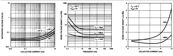
*Figure 7. Saturation Voltage vs. Collector Current*
