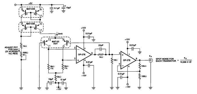
Figure 13. MAT03 Voltage Noise Measurement Circuit
