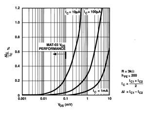
Figure 17b. Current Matching Accuracy % vs. Offset Voltage
