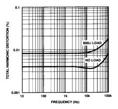
Figure 14b. Super Low Noise Amplifier—Total Harmonic Distortion
