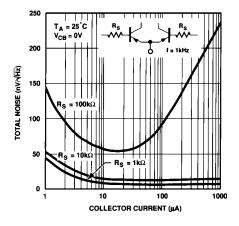
Figure 10. Total Noise vs. Collector Current
