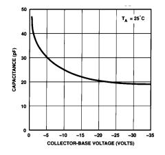
Figure 11. Collector-Base Capacitance vs. V<sub>CB</sub>
