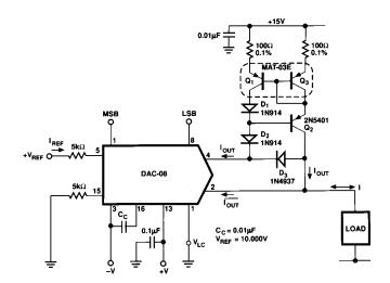
Figure 18. Digitally Programmable Bipolar Current Pump
