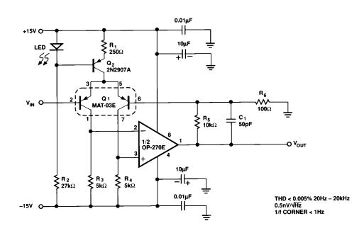
Figure 15. Low Noise Microphone Preamplifier
