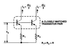
Figure 17a. Current Matching Circuit
