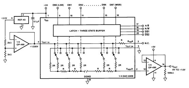
Figure 8. Unipolar Supply, Voltage Output DAC Operation
