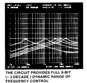
Figure 10. Programmable Active Filter Band-Pass Frequency Response
