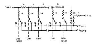
Figure 1. Simplified D/A Circuit of DAC8408
