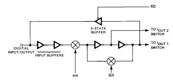
Figure 5. Digital Input/Output Structure
