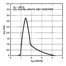
Supply Current vs. Logic Level
