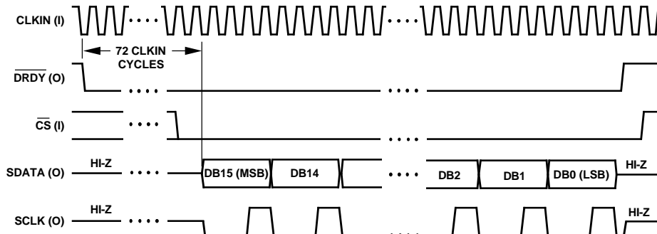
Figure 19. SSC Mode Showing Data Timing Relative to SCLK
