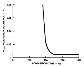
Figure 1. V<sub>OUT</sub> Settling vs. Acquisition Time
