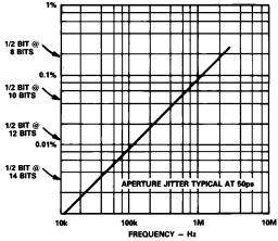
Figure 6. Error Magnitude vs. Frequency
