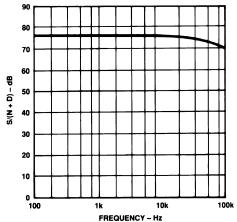
Figure 8. Signal/(Noise and Distortion) vs. Frequency
