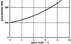
Acquisition Time (to 0.01 %) vs. Input Step Size
