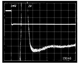
Figure 2. Typical AD684 Hold Mode
