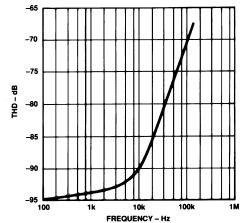
Figure 7. Total Harmonic Distortion vs. Frequency
