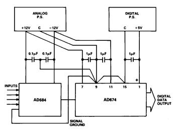
Figure 4. Basic Grounding and Decoupling Diagram
