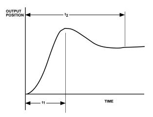
Figure 7. AD2S81A/AD2S82A Small Step Response
