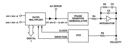
Figure 3. AD2S81A/AD2S82A Functional Diagram
