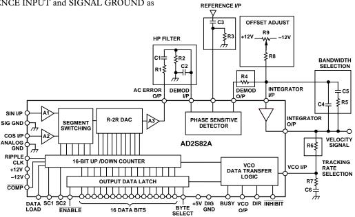
Figure 1a. AD2S82A Connection Diagram
