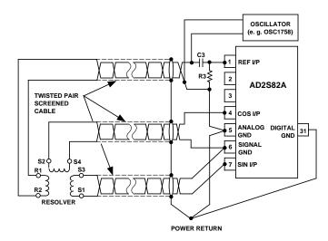
Figure 8. Connecting the AD2S82A to a Resolver
