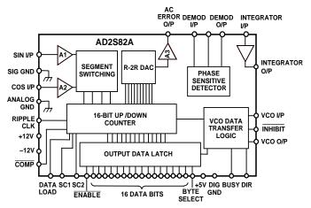
An analog signal proportional to velocity is also available and can be used to replace a tachogenerator.
