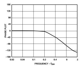
Figure 6. AD2S81A/AD2S82A Phase Plot
