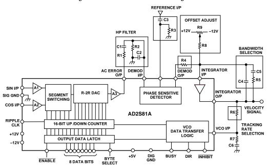
Figure 1b. AD2S81A Connection Diagram
