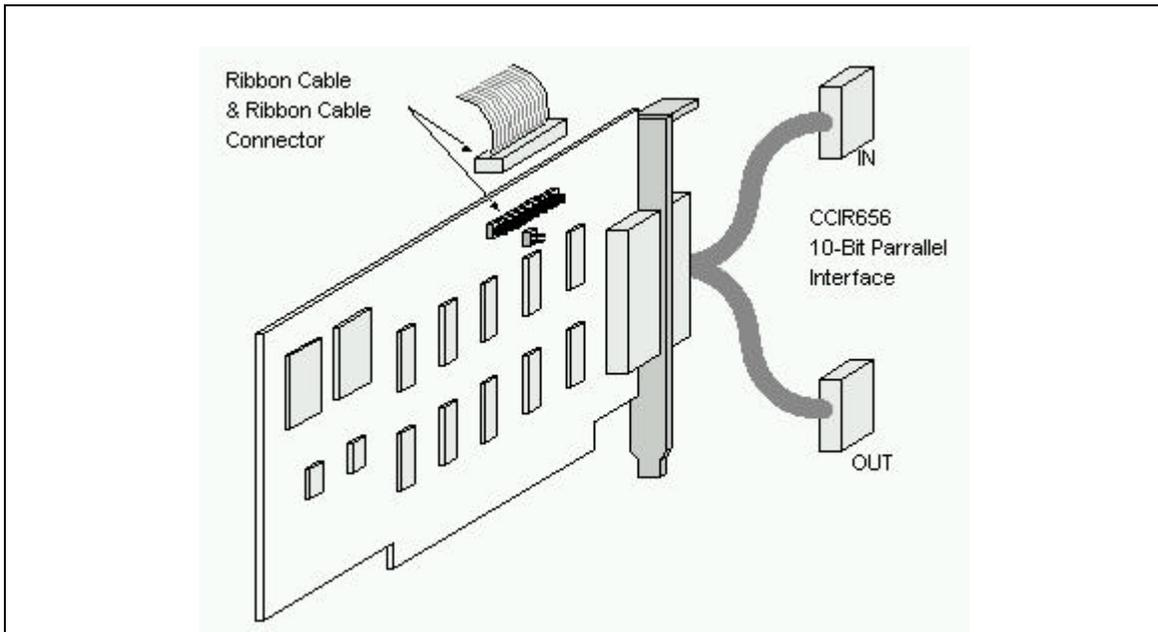
*CCIR656 ECL Interface ISA Board w/ D-Shell Breakout Cable*
