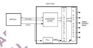
Figure 32 PLL and 4xOversampling block diagram
