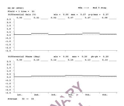
Figure 121. NTSC Differential Gain and Phase Measurement
