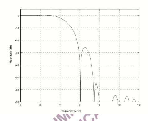
Figure 8 Luma NTSC Low Pass Filter (4xOversampling)
