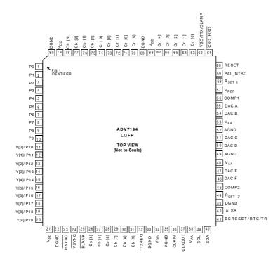
Figure 5. Pin Configuration ADV7194
