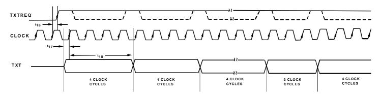
Figure 3. Teletext Timing Diagram
