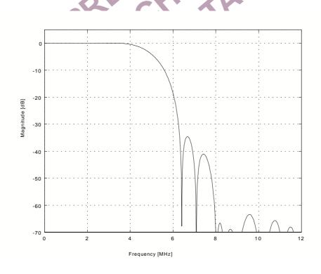
Figure 9 Luma PAL Low Pass Filter (4xOversampling)
