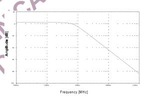
Figure 102. Output Filter Plot for 2xOversampling filter
