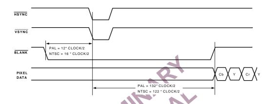
Figure 45. Timing Mode 2 Even to Odd Field Transistion Master/Slave
