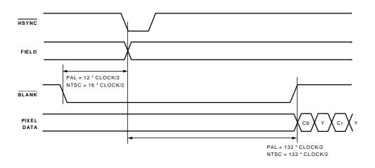
Figure 42. Timing Mode 1 Odd/Even Field Transitions Master/Slave
