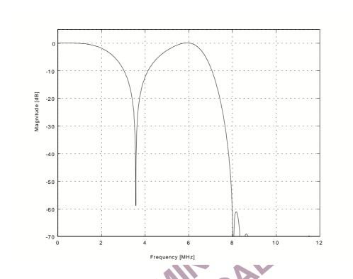
Figure 10 Luma NTSC Notch Filter (4xOversampling)
