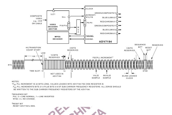
Figure 35. RTC Timing and Connections
