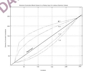
Figure 92 Signal Input (Ramp) and selectable Gamma Output
