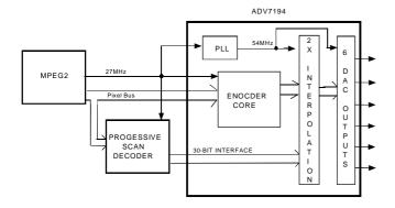
Figure 31. Block diagram of using the ADV7194 in Progressive Scan Mode
