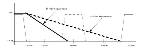
Figure 104. Output Filter Requirements in 4xOversampling Mode
