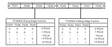
Figure 72. Teletext Control Register
