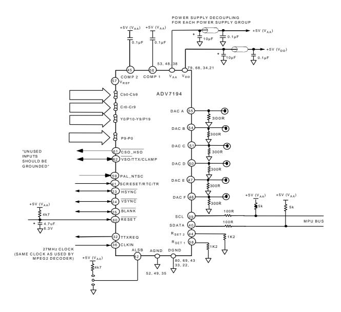
Figure 94. Recommended Analog Circuit Layout
