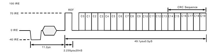
Figure 96. CGMS Waveform diagram
