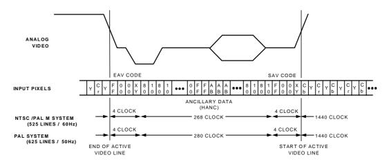
Figure 36. Timing Mode 0 (Slave Mode)
