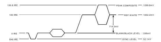
Figure 111. NTSC Composite Video Levels
