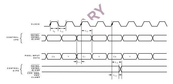
Figure 2. Pixel and Control Data Timing Diagram
