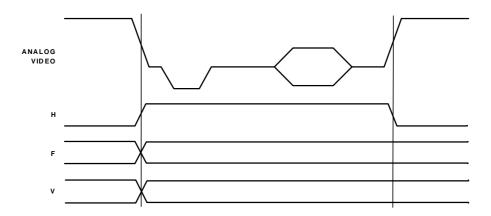
Figure 39. Timing Mode 0 Data Transitions (Master Mode)
