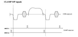
Figure 27 Clamp output timing
