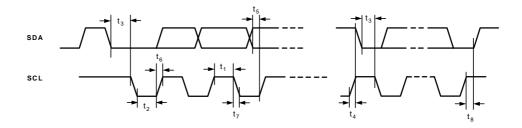
Figure 1. MPU Port Timing Diagram
