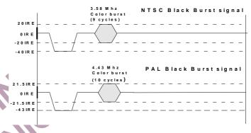
Figure 62 Black Burst signals for PAL and NTSC standards
