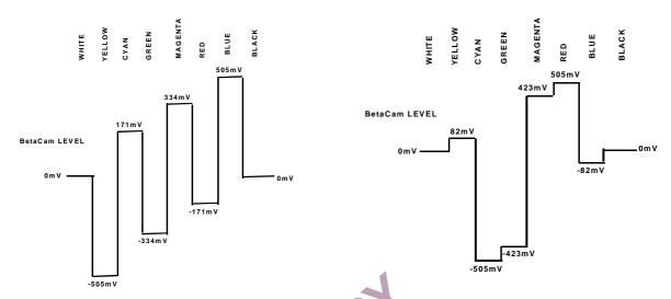
Figure 133. NTSC 100% Color Bars No Pedestal U Levels Figure 134. NTSC 100% Color Bars No Pedestal V Levels
