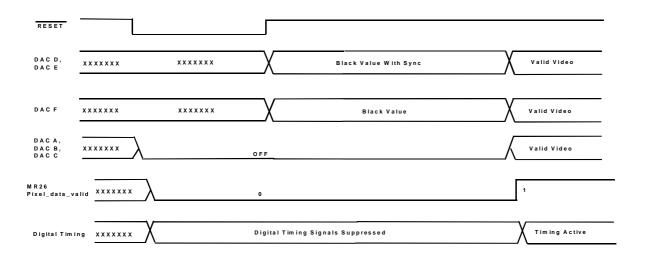
Figure 34. RESET Sequence Timing Diagram
