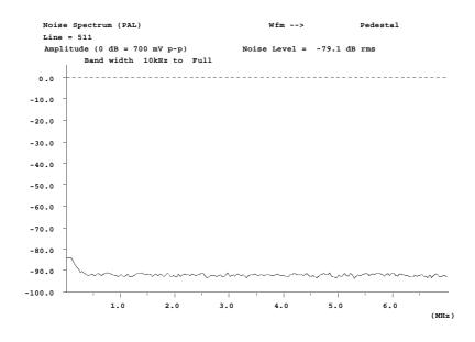
Figure 130. PAL Noise Spectrum - Pedestal
