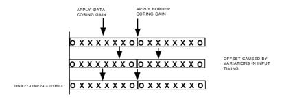
FIGURE 90 DNR 27-24, BLOCK OFFSET CONTROL
