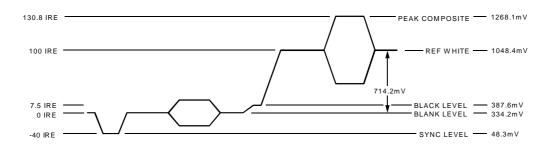
Figure 107. NTSC Composite Video Levels
