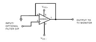
Figure 106. Recommended DAC Output Buffer using an OP-amp
