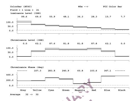
Figure 119. NTSC Color Bars Measurement
