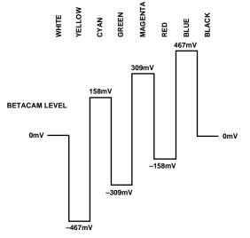
Figure 58. NTSC 100% Color Bars with Pedestal U Levels
