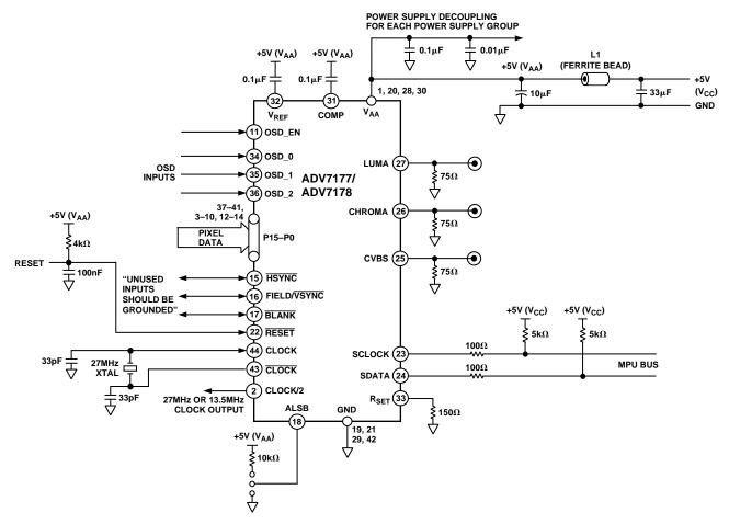
Figure 43. Recommended Analog Circuit Layout
