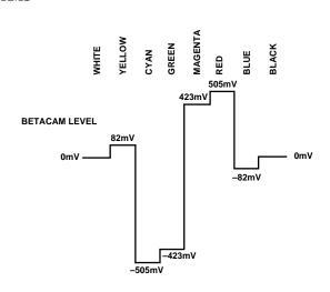
Figure 60. NTSC 100% Color Bars No Pedestal V Levels
