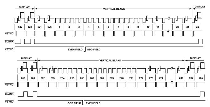
Figure 21. Timing Mode 2 (NTSC)
