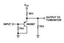
Figure 68. Recommended Output DAC Buffer
