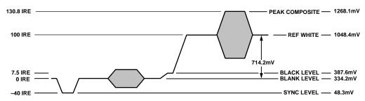
Figure 45. NTSC Composite Video Levels
