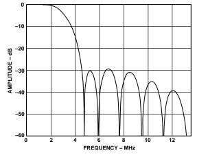
Figure 10. PAL Notch Filter
