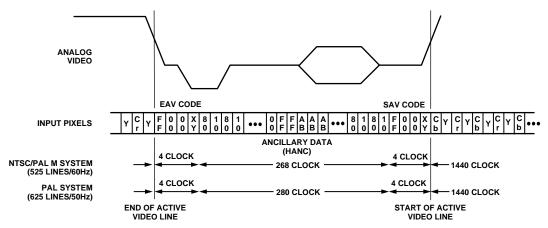
Figure 14. Timing Mode 0 (Slave Mode)
