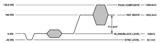
Figure 49. NTSC Composite Video Levels
