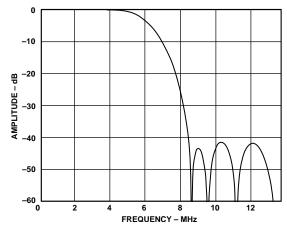
Figure 11. NTSC/PAL Extended Mode Filter
