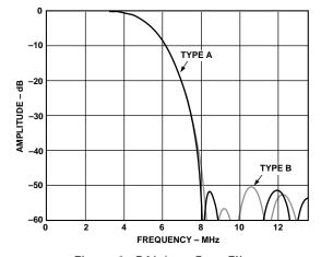
Figure 9. PAL Low-Pass Filter
