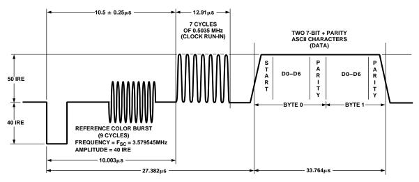
Figure 44. Closed Captioning Waveform (NTSC)
