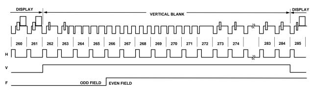
Figure 15. Timing Mode 0 (NTSC Master Mode)
