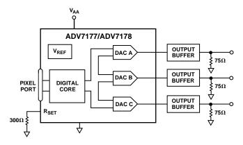
Figure 67. Output DAC Buffering Configuration
