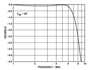
Figure 66. Output Filter Plot Close Up
