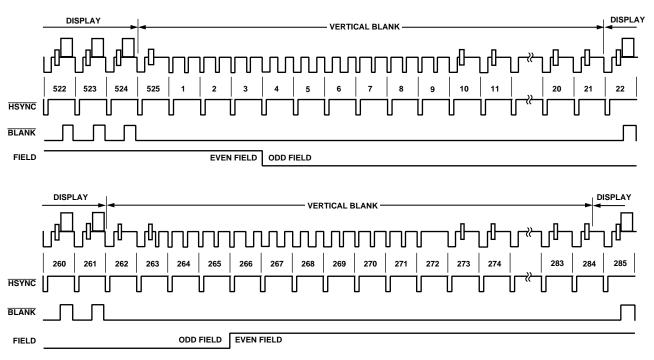
Figure 18. Timing Mode 1 (NTSC)
