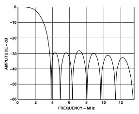
Figure 8. NTSC Notch Filter
