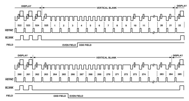
Figure 25. Timing Mode 3 (NTSC)
