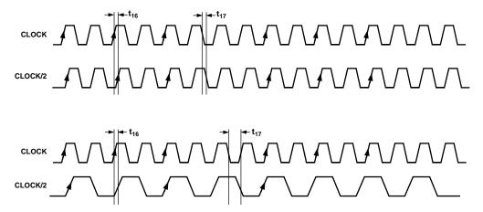
Figure 3. Internal Timing Diagram
