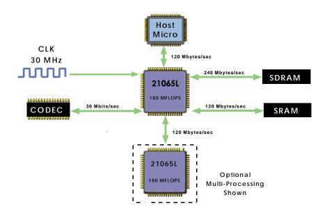
SHARC DSPs provide superior system performance to a wide range of real-time, embedded applications. The ADSP-21065L uses multiple buses to create high-speed thoroughfares between the core, I/O peripherals, internal dual-ported memory and external synchronous DRAM.
