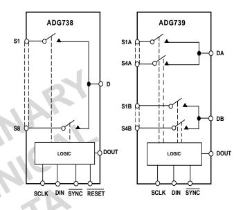
All channels exhibit break before make switching action preventing momentary shorting when switching channels. The ADG738 and ADG739 are available in 16 lead TSSOP package.
