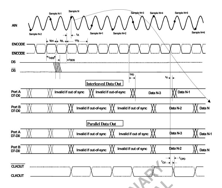
Figure 1. Timing Diagram – Dual Channel Mode with Clock Doubler Disabled.
