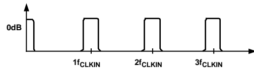
Figure 27a. Digital Filter Frequency Response
