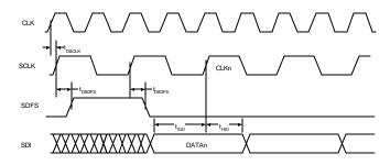
Figure X. Serial Port Switching Characteristics.
