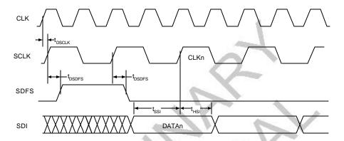
Figure X. Serial Port Switching Characteristics.
