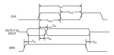
Figure X. Parallel Output Switching Characteristics.
