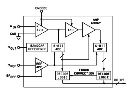
FIGURE 3. Block diagram.
