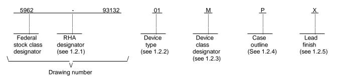
1.2.1 <u>RHA designator</u>. Device classes M, B, and S RHA marked devices shall meet the MIL-M-38510 specified RHA levels and shall be marked with the appropriate RHA designator. Device classes Q and V RHA marked devices shall meet the MIL-I-38535 specified RHA levels and shall be marked with the appropriate RHA designator. A dash (-) indicates a non-RHA device.
