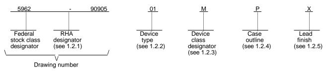
1.2.1 <u>RHA designator</u>. Device classes M, B, and S RHA marked devices shall meet the MIL-M-38510 specified RHA levels and shall be marked with the appropriate RHA designator. Device classes Q and V RHA marked devices shall meet the MIL-I-38535 specified RHA levels and shall be marked with the appropriate RHA designator. A dash (-) indicates a non-RHA device.
