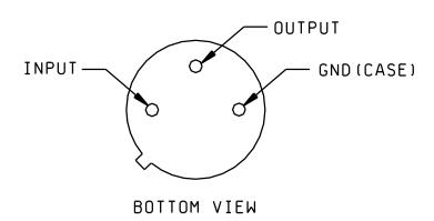
FIGURE 2. <u>Terminal connections</u>.
