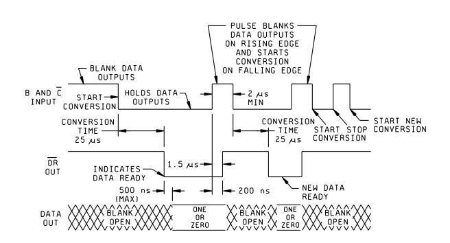
FIGURE 2. Timing waveforms.
