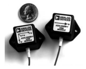
All that is required to use these modules is a +5 volt power supply. The module should be attached (i.e., screwed or glued down) securely to the object being measured, taking care that the axis of sensitivity, indicated by the large arrow on the top of the module, is aligned with the expected acceleration.
