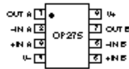
8-Lead Narrow-Body SO (S Suffix)
