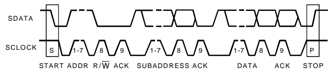
Figure yy. Bus Data Transfer
