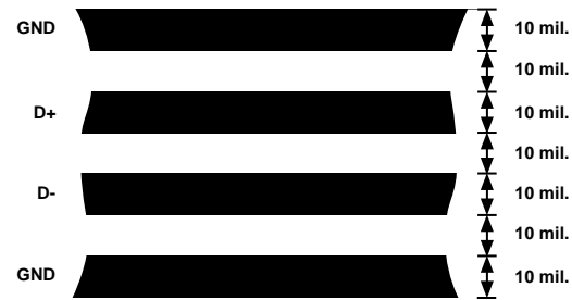
Figure 5. Arrangement of Signal Tracks
