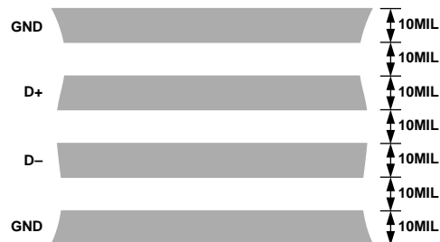
Figure 12. Arrangement of Signal Tracks
