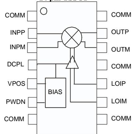
The open-collector differential outputs may be used to drive a differential IF signal chain or may be converted to a single-ended signal through the use of a matching network or transformer. The outputs may swing  $\pm 1$  V centered on the VPOS supply voltage.
