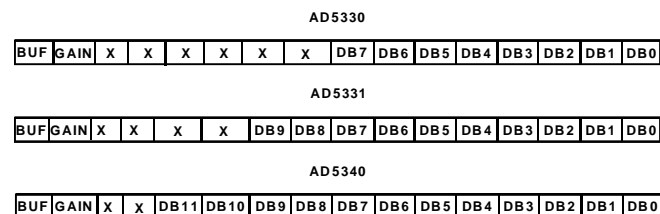
Figure 8. Data format for GAIN and BUF data on a 16-bit Bus
