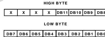
Figure 7. Data Format For AD5341
